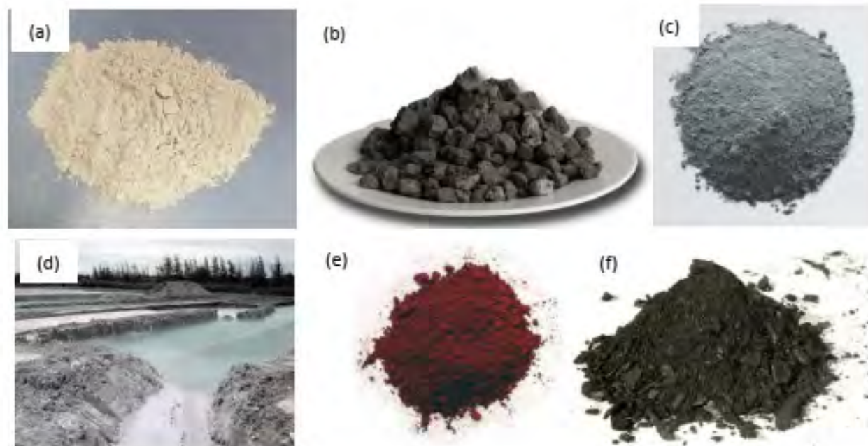
Industrial by-products and wastes to be investigated in this study (a) GGBS; (b) steel slag; (c) coal fly ash; (d) CCR; (e) red mud; and (f) biochar
