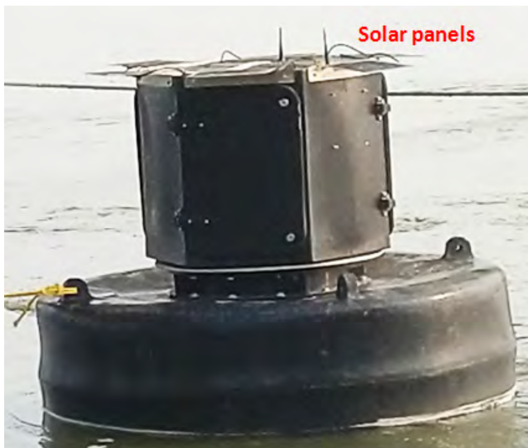
Autonomous Aquatic Observatory (AAO) with Solar panels deployed in River Ganga (Kanpur, India)
